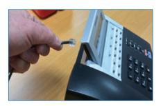
VOICE Support for 1, 2 or 3-pair RJ11/12 telephone cable testing
